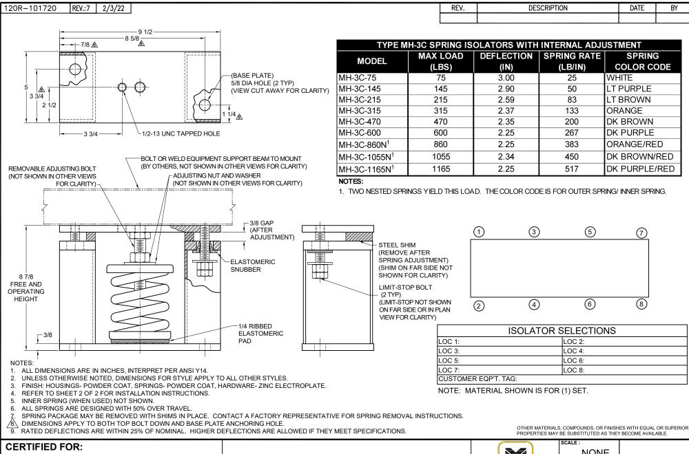
NONE MODEL MH-3C 75-1165 LBS. JOB NAME: SHEET: SPRING ISOLATORS WITH 1 OF 2 CUSTOMER: INTERNAL ADJUSTMENT GROUP DRAWING NO REVISION CUSTOMER P.O.: 3 INCH DEFLECTION THE POWER OF TOGETHER' Bloomingdale, NJ 07403 SALES ORDER: Houston, TX 77041
